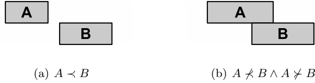
Figure 7.4: Two examples demonstrating the partial order on intervals. Intervals that overlap are not related.
